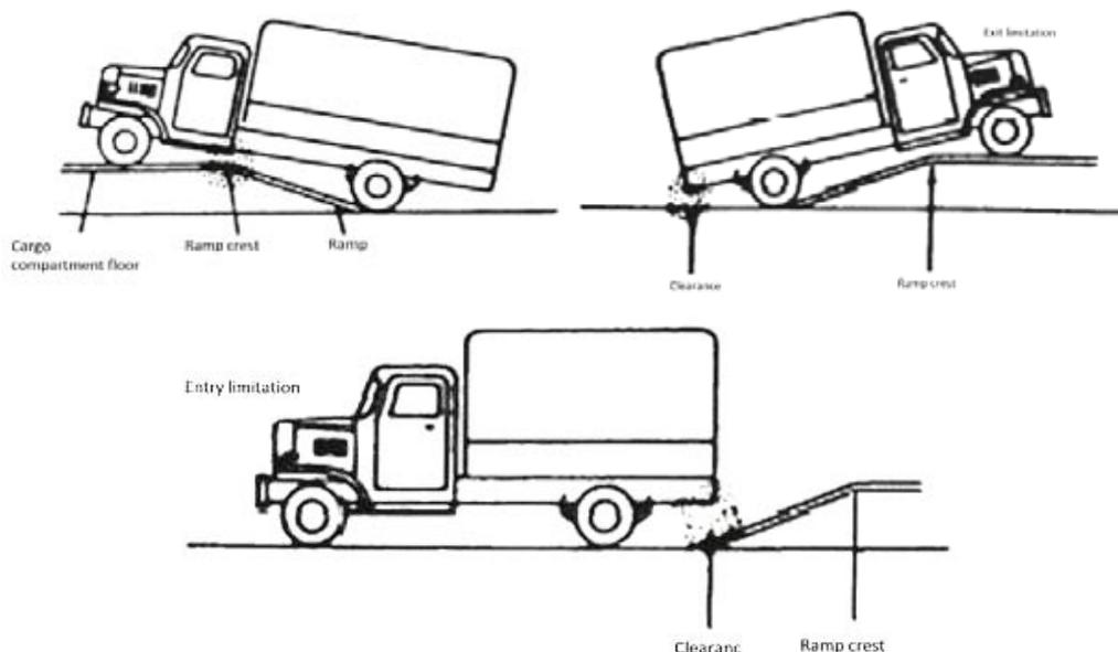
**Fig. 3. Front and rear overhang and ramp crest angle that constitute limitations of entry into the cargo hold [7]**
