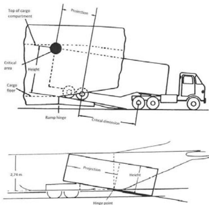
**Fig. 4. Load height limitations resulting from overhang distance during loading [7]**
