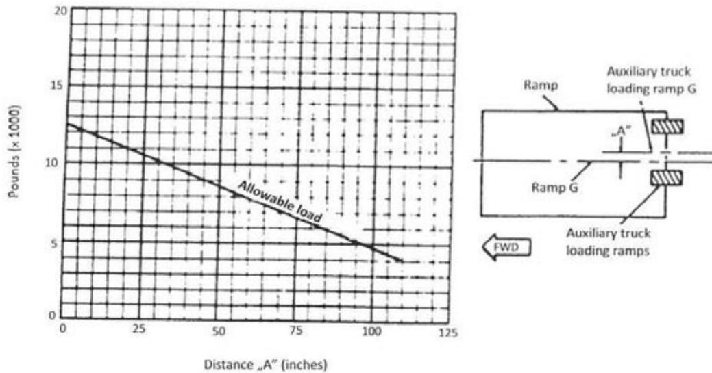
**Fig. 5. Permissible maximum offset position of load centre of gravity affecting the transverse stability of the aircraft (graph for C-130) [5]**
