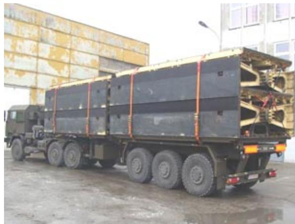
**Fig. 10. View of carrier vehicle with main MS-40 bridge spans**
