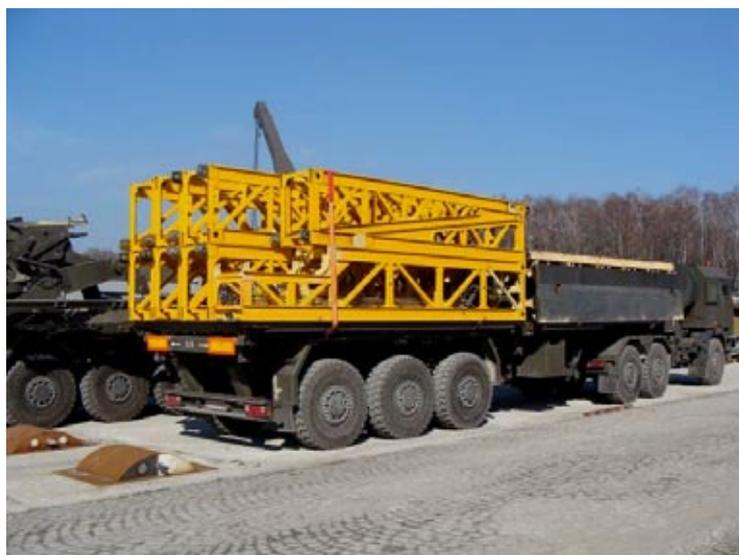
**Fig. 11. Auxiliary spans of MS-40 bridge on carrier vehicle**
