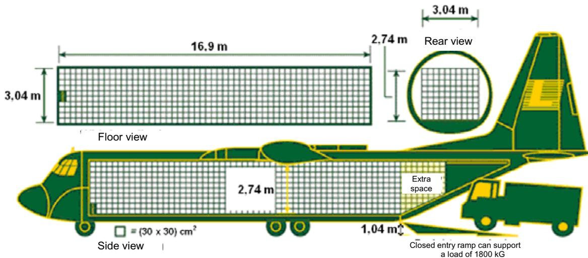
**Fig. 6. Dimensions of the loading space of the C-130J-30 Hercules transport aircraft [9]**
