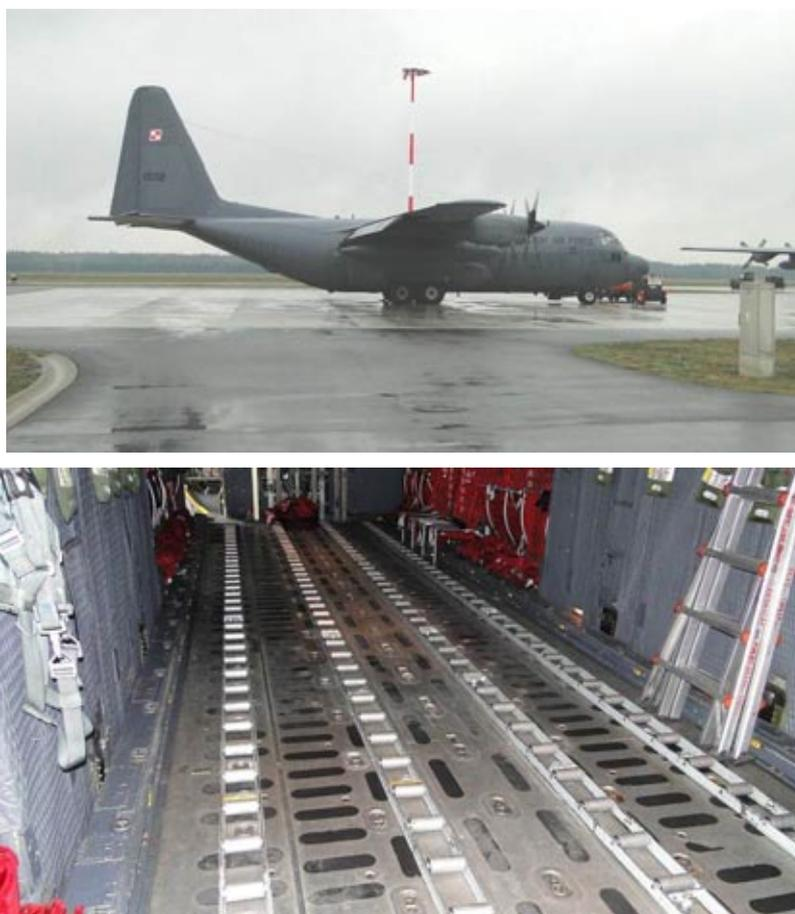
**Fig. 8. C-130E Hercules transport aircraft. General view and cargo hold interior**
