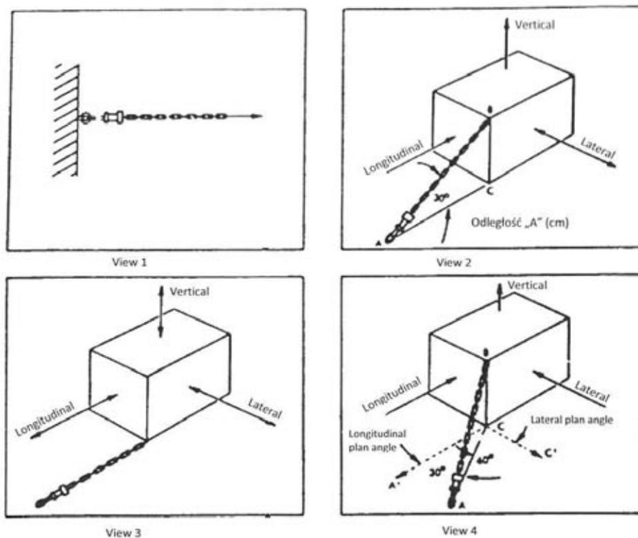
**Illustration of the effect of oblique arrangement of stays on the forces in the main directions of reaction (at reduced strength of rope and anchoring system), and of the transfer of loads resulting from flight instability [8]**
