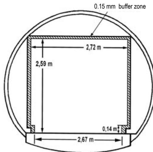
**Fig. 1. Illustration of the free loading space limitations in a C-130 transport aircraft [7]**
