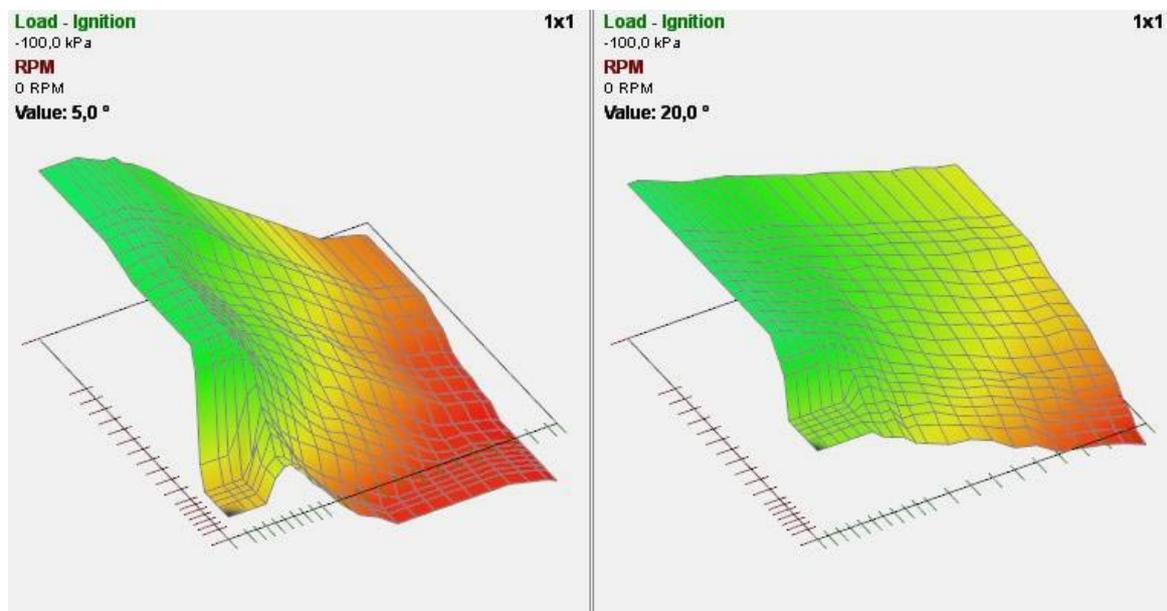
**Fig. 3. Ignition advance angle vs. load and speed in a 4G63T engine with rated output of 206 kW and 309 kW**
