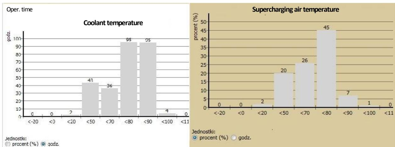
**Fig. 9. Graphs stored in the memory of a controller of a Rosomak APC**
