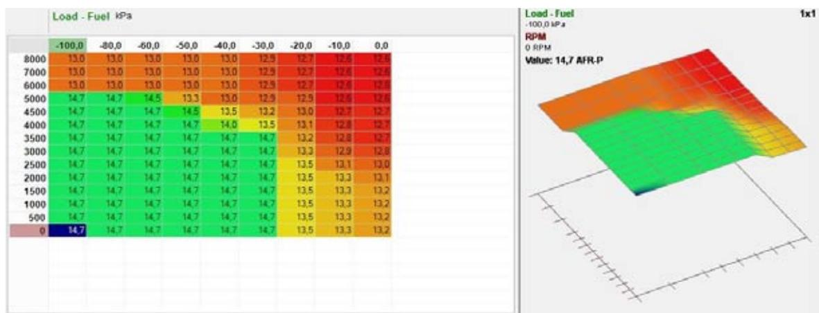
**Fig. 2. Characteristics of optimum air to fuel ratio for a spark ignition engine depending on load and speed of the engine (AFR = 14.7, corresponds to  $\lambda=1$ )**
