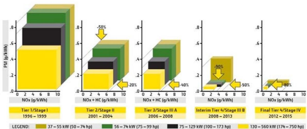
Fig. 1. Comparison of exhaust gas emission limits for utility vehicles between 1996 and 2015 [3]
