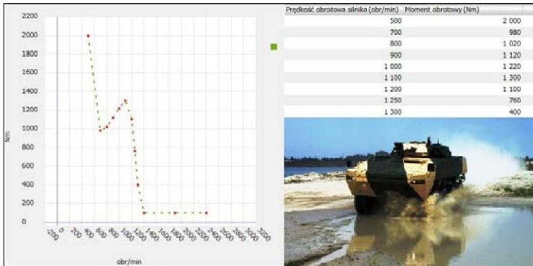
**Fig. 5. Emergency torque limiting function**
