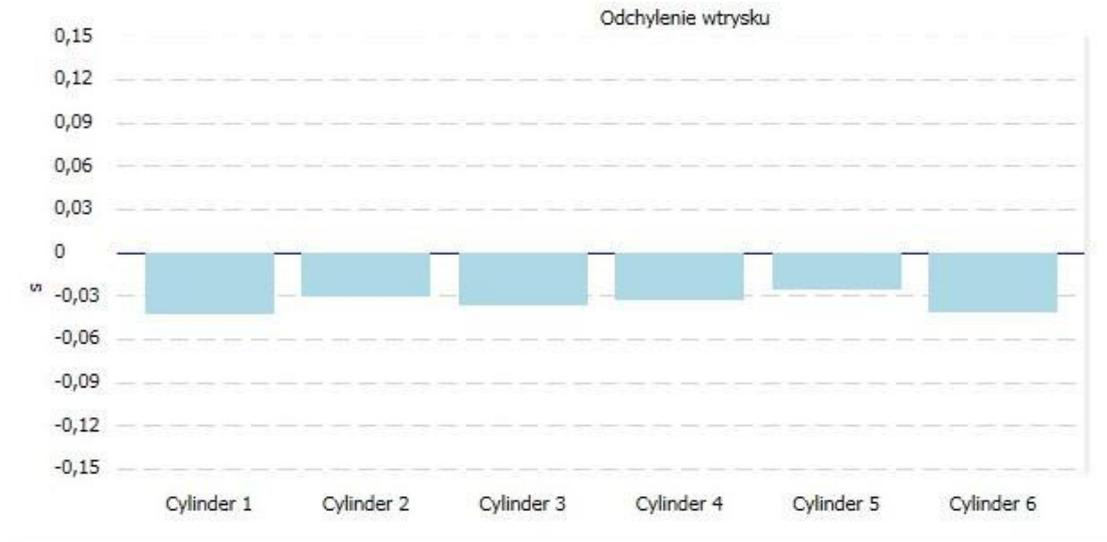
**Fig. 8. Maintenance program display – fuel injection time deviations for individual cylinders**
