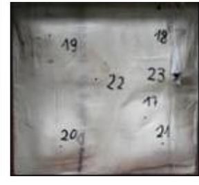
**Fig. 4. Armour panel with  $\text{B}_4\text{C}$  ceramics (thickness: 20mm, weight:  $32\text{kg/m}^2$ ), front and back**
