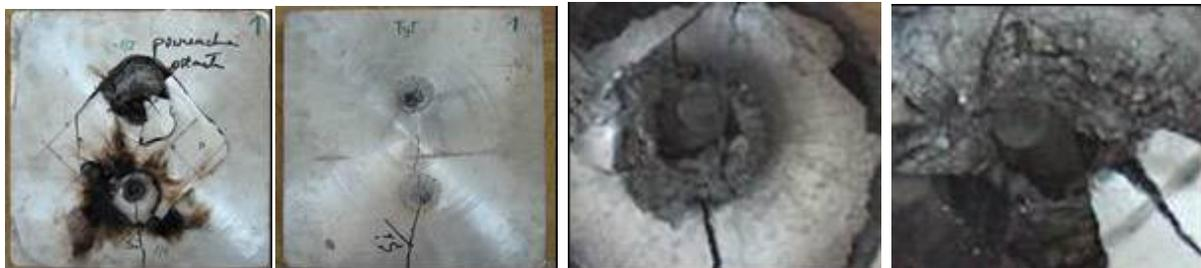
**Fig. 3. Front and rear view of panel no. 8 hit with two projectiles and view of projectile lodged in panel**
